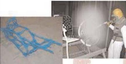
Our 10 ft x 10 ft x 25 ft media blasting booth allows for large items such as panels and frames to be properly prepared for powder coating.
