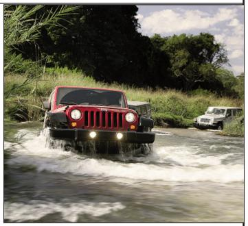
Shortly after crossing, the Jeep literally died. After getting it back to the dealership, the owner learned that the engine had extensive damage from water in the cylinders. The result was a cracked block, broken connecting rods and damaged cylinder heads. Bikes and ATVs can also be damaged when hot driveline components meet cold water. Continued on page 16
